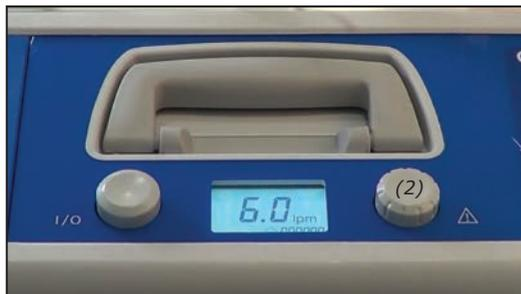
1. Press the adjustment regulator (2) for at least 2 seconds.
