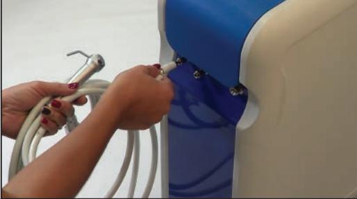
*Connect the oxygen hose to the outlet connector on one side and to the diffusers on the other side.*
