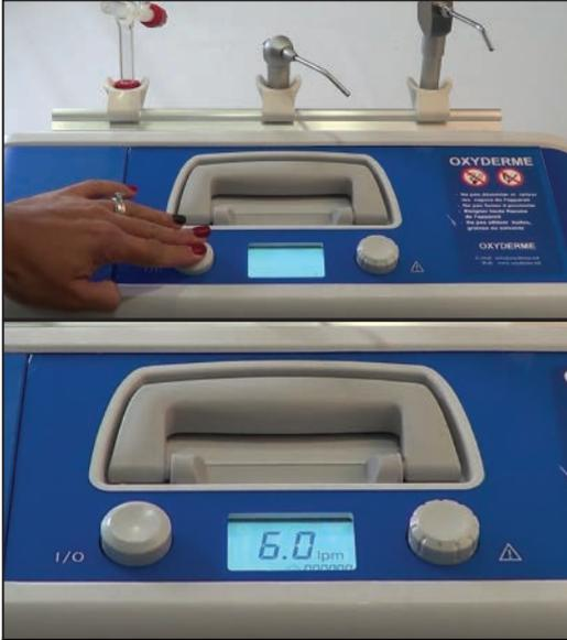
Start the unit by activating the mains switch (1) on top of the unit.
